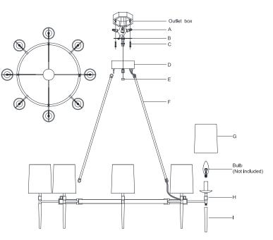
10. Connect the Hot (smooth edge, markings, or black) fixture wire with the Hot (usually black) wire from your outlet box using wire nut (A).
