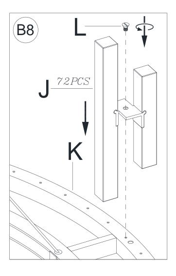
Loosen the Set Screws (L), then place the Brackets (J) onto the Light Fixture (K) and secure the Brackets (J) by tightening Set Screws in a clockwise (L)
