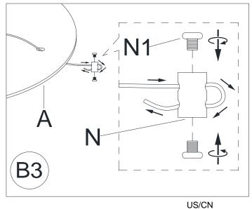
Replace the Lock connector (N) to the end of the safety cable and secure by inserting Set Screws (N1).
