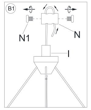
Loosen set screws (N1), pull out the safety cable from lock connector (N).
