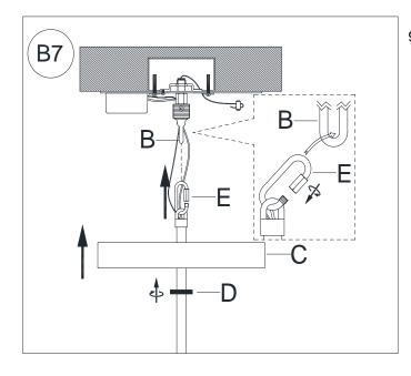
9. Attach Hanging loop (E) to Mounting Loop (B) and secure by closing the hex nut on Hanging Loop (E). Attach the Canopy (C) onto the Mounting Plate (A) then secure the Canopy (C) by turning the Canopy Nut (D) in a counter-clockwise direction.
