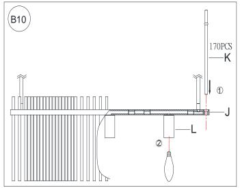
10. Insert the specified light bulbs into the Socket (L). DO NOT EXCEED THE SPECIFIED WATTAGE. Insert the Crystal Bars (K) into the holes on Light Fixture (J)
