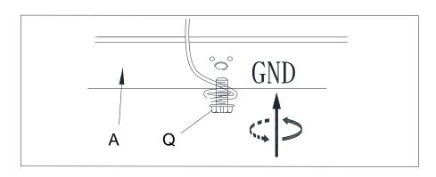
If the junction box DOES NOT have a GROUND WIRE, wrap the fixture's bare ground wire around the Green Ground Screw (Q) and insert the screw into the Mounting Plate (A), marked as "GND", and tighten screw to secure the wire.
