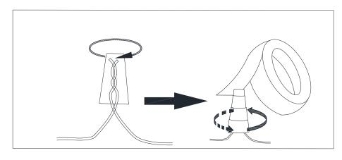
Connect the GROUND FIXTURE WIRE to the GROUND J-BOX WIRE using the Plastic Wire Nut Connector (P) and wrap the connection with electrical tape. Be sure that no wire strands are exposed.
