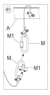
7. With the help of another person to hold the weight of the lighting fixture, unscrew the Closable Link Screw Cap (M1) from the Closable Link (M), attach each Closable Link (M) from the Mounting Plates (A) onto each Closable Link (M) from the Canopy (C). Tighten each Closable Link Screw Cap (M1) as shown in diagram. Now the lighting fixture is supported by the steel wires.
