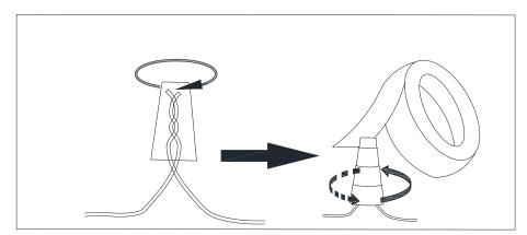
Connect the NEUTRAL FIXTURE WIRE to the NEUTRAL J-BOX WIRE first and then connect the HOT FIXTURE WIRE to the HOT J-BOX WIRE using the Plastic Wire Nut Connectors (P). Wrap these connections with electrical tape. Be sure that no wire strands are exposed.
