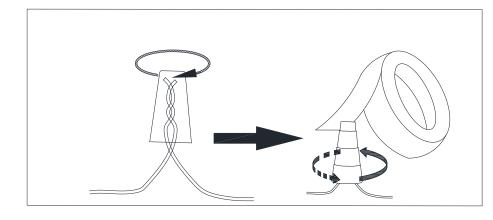
Connect the GROUND FIXTURE WIRE to the GROUND J-BOX WIRE using the Plastic Wire Nut Connector (P) and wrap the connection with electrical tape. Be sure that no wire strands are exposed.
