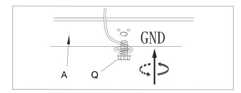
If the junction box DOES NOT have a GROUND WIRE, wrap the fixture's bare ground wire around the Green Ground Screw (Q) and insert the screw into the Mounting Plate (A), marked as "GND", and tighten screw to secure the wire.
