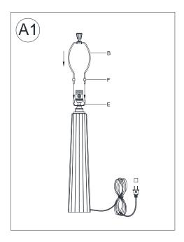
Raise the Harp Caps (F) and insert the bottom ends of Harp (B) into the Saddle (E).
