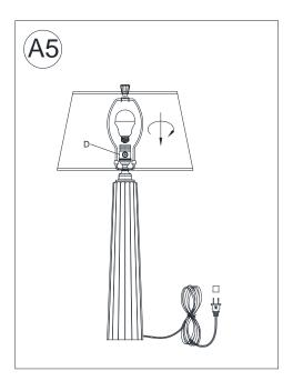
Insert the specified light bulb into the Socket (D).DO NOT EXCEED THE SPECIFIED WATTAGE.
