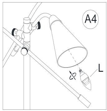
Insert the specified light bulbs (L) into the Sockets (F). DO NOT EXCEED THE SPECIFIED WATTAGE.
