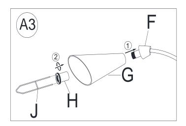
Attach Glass Shades (G) to the threaded portion of Sockets (F) and secure with Socket Rings (H). Tighten with Fork Wrench (J).
