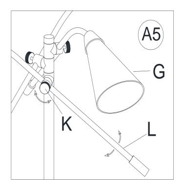
If need, loosen Adjustment Knobs (K), swing Lamp Arms (L) to adjust Glass Shades (G) to desired position and secure by tightening Adjustment Knobs (K).
