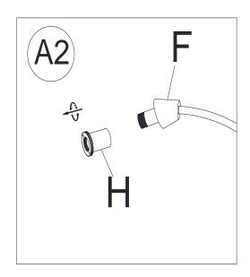
Remove Socket Rings (H) from Sockets (F) by turning clockwise direction.
