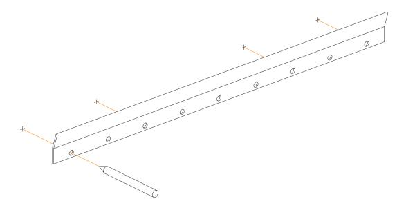
3. To ensure proper installation of the toggles, align the pointed end of the ITW Toggle (C) against the marks from previous step. Use Philips Head Screwdriver to rotate the ITW Toggle (C) clockwise as you push it lightly to the wall. The ITW Toggle (C) will self-drill and thread into the sheetrock as it is rotated. Continue rotating until the flange of the ITW Toggle (C) meets flush with the wall surface. Repeat this step for the rest of the ITW Toggle (C).
