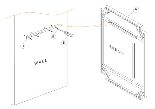
5. Hang the Mirror Frame (A) by aligning the metal plate found at the back to the installed Hanging Bracket (D) on the wall either vertically or horizontally.
