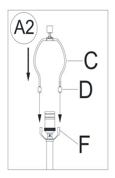
Raise the Harp Caps (D) and insert the bottom ends of Harp (C) into the Saddles (F)
