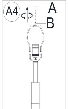
Unscrew the Finial (A) from the Harp Top (B) by turning counter-clockwise direction.
