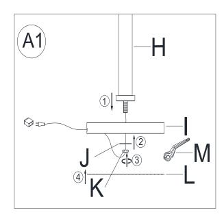
1. Fully insert the bottom threaded nipple of the Lamp Pole (H) into the center hole of the Lamp Base (I) until the threaded portion of the Lamp Pole (H) is exposed on the bottom side of Lamp Base (I). Position the Spring Washer (J) first and then the Hex Nut (K) onto the extended threaded portion from the Lamp Pole (H), tighten the Hex Nut (K) to secure the Lamp Pole (H) onto the Lamp Base (I) until tight using a Wrench (M).
