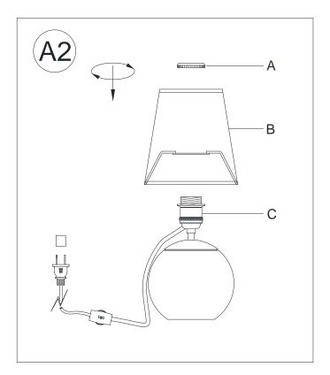
Place the lampshade(B) to the socket(C) and tighten with socket ring(A)
