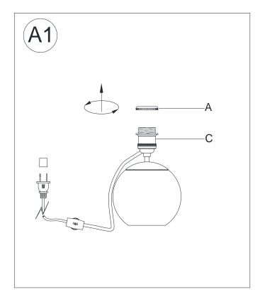
Remove the socket ring(A) from socket(C).
