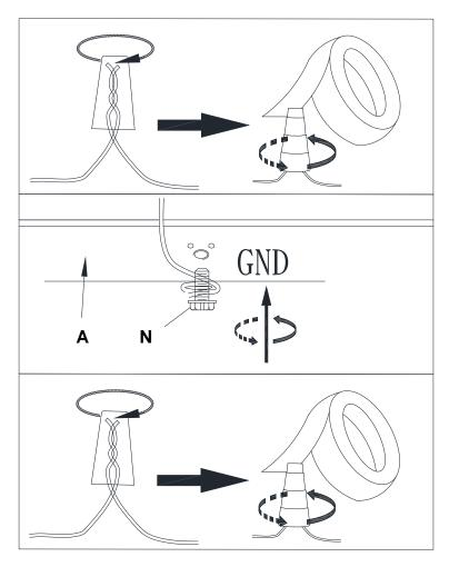
Connect the GROUND FIXTURE WIRE to the GROUND J-BOX WIRE using the Plastic Wire Nut Connector (P) and wrap the connection with electrical tape. Be sure that no wire strands are exposed.
