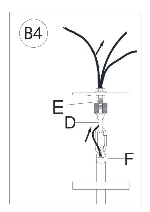
Feed the fixtures power cord and bare ground wire and Steel Cable through Hanging Loop (F) and Threaded Tube (E).
