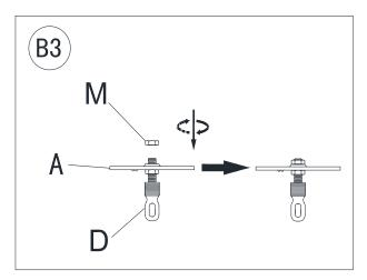
Position the Lock Washer (L) first and then the Hex Nut (M) onto the top end of Threaded Tube (E). Tighten the Hex Nut (M) until tight using pliers so that the Hanging Loop (D) is now firmly secured to the middle of the Mounting Plate (A).
