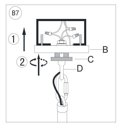
Slide the Canopy (B) upward along the Connection Tube (G) with the upper rim of the canopy pressed gently against the ceiling surface. Position the Canopy Nut (C) against the Fixture Loop (D) and rotate the nut clockwise to engage it with the threaded portion of the Fixture Loop (D) until secure. Do not over tighten this nut.
