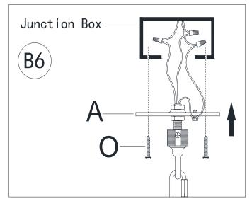
Attach the Mounting Plate (A) onto the junction box using Mounting Screws (O).
