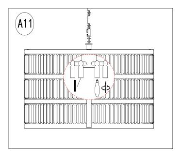
Insert eight (8) **60-watt maximum TYPE B (candelabra) standard light bulbs** (not included) or eight (8) **13-watt compact fluorescent light bulbs**(not included) into the Sockets (I). DO NOT EXCEED THE SPECIFIED WATTAGE.
