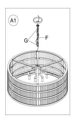
3. (See A2) Weave the fixtures 2 wire power cord and bare ground wire through every other loop to the top of Chain (F).
