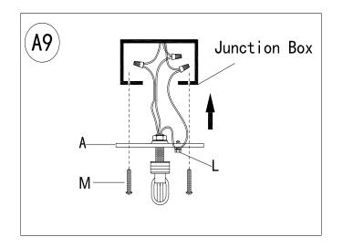
Attach the Mounting Plate (A) onto the junction box using two 10-24 Mounting Screws (M).
