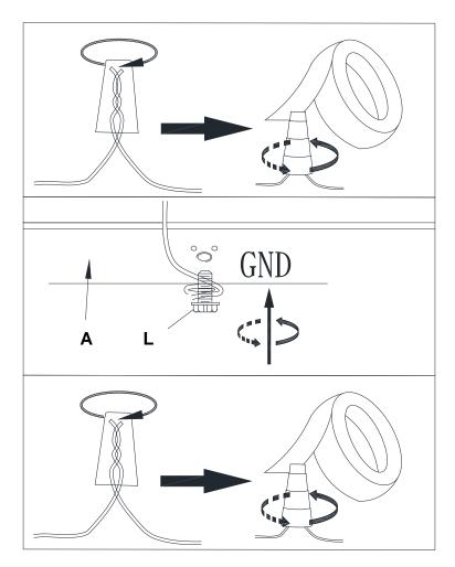
Connect the GROUND FIXTURE WIRE to the GROUND J-BOX WIRE using the Plastic Wire Nut Connector (N) and wrap the connection with electrical tape. Be sure that no wire strands are exposed.
