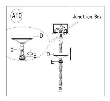
Slide the Canopy (D) upward along the Chain (F) with the upper rim of the canopy pressed gently against the ceiling surface. Position the Canopy Nut (E) against the Mounting Loop (C) and rotate the nut clockwise to engage it with the threaded portion of the Mounting Loop (C) until secure. Do not over tighten this nut.
