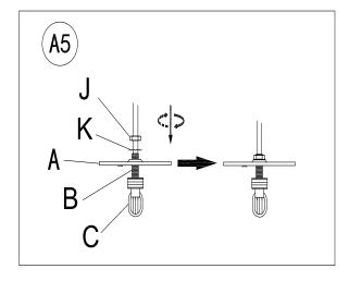
Position the Lock Washer (K) first and then the Hex Nut (J) onto the top end of Threaded Tube (B). Tighten the Hex Nut (J) until tight using pliers so that the Hanging Loop (C) is now firmly secured to the middle of the Mounting Plate (A).
