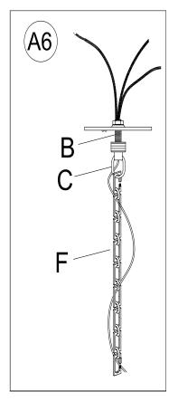
Feed the fixtures power cord and bare ground wire and Safety Steel Cable through Mounting Loop (C) and Threaded Tube (B).
