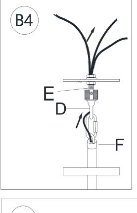
Feed the fixtures power cord and bare ground wire and Steel Cable through Hanging Loop (F) and Threaded Tube (E).
