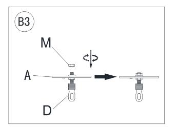
Position the Lock Washer (L) first and then the Hex Nut (M) onto the top end of Threaded Tube (E). Tighten the Hex Nut (M) until tight using pliers so that the Hanging Loop (D) is now firmly secured to the middle of the Mounting Plate (A).
