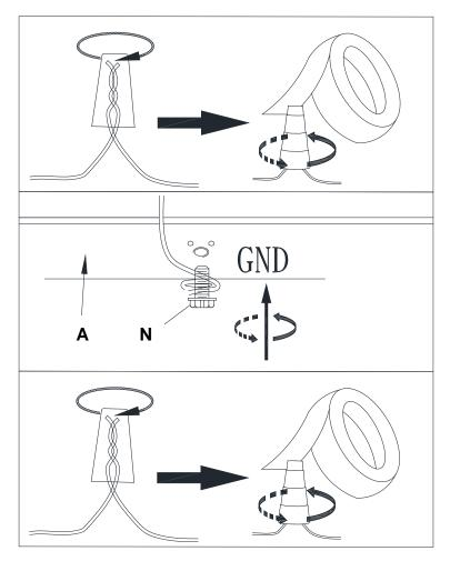
Connect the GROUND FIXTURE WIRE to the GROUND J-BOX WIRE using the Plastic Wire Nut Connector (P) and wrap the connection with electrical tape. Be sure that no wire strands are exposed.
