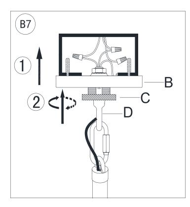
Slide the Canopy (B) upward along the Connection Tube (G) with the upper rim of the canopy pressed gently against the ceiling surface. Position the Canopy Nut (C) against the Fixture Loop (D) and rotate the nut clockwise to engage it with the threaded portion of the Fixture Loop (D) until secure. Do not over tighten this nut.
