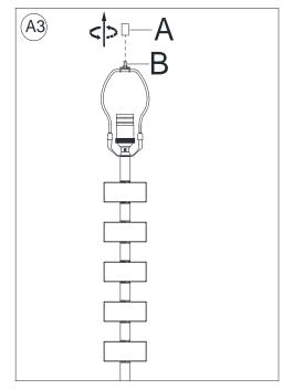
Unscrew the Finial (A) from the Harp Top (B) by turning counter-clockwise direction.
