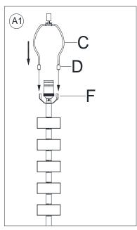
Raise the Harp Caps (D) and insert the bottom ends of Harp (C) into the Saddles (F)
