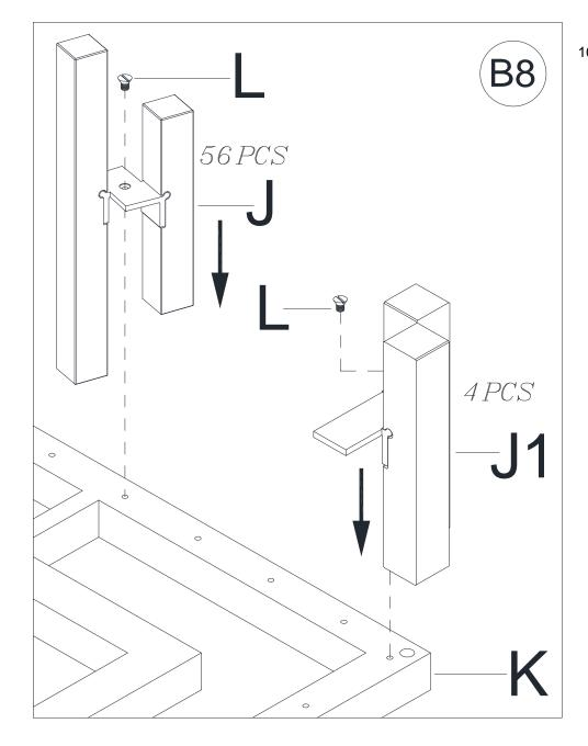
10. Loosen the Set Screws (L), place the Brackets (J1) onto the 4 corner of Light Fixture (K) and place the Brackets (J) onto the Light Fixture (K) and secure the Brackets (J) and (J1) by tightening Set Screws (L) in a clockwise.
