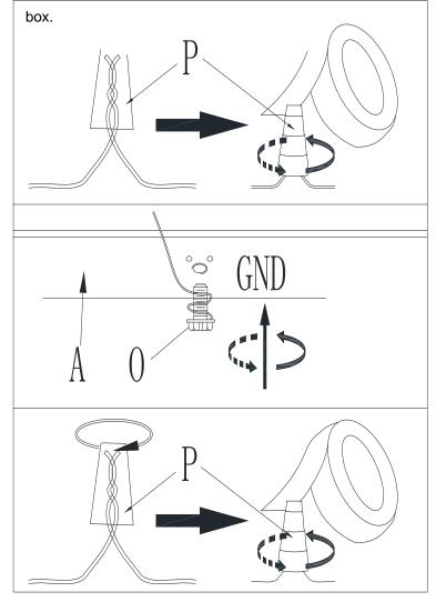
Connect the GROUND FIXTURE WIRE to the GROUND J-BOX WIRE using the Plastic Wire Nut Connector (P) and wrap the connection with electrical tape. Be sure that no wire strands are exposed.
