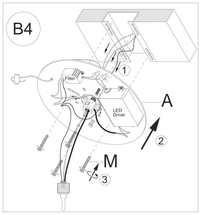
5. Gently pull existing wire down from the ceiling junction box and through the center hole on mounting plate (A)6. Attach Mounting Plate (A) to ceiling junction box with Mounting Screws (M) provided.
