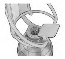
Add the Filling Cap (with O-Ring in place) and screw on the Cap Collar. Be careful not to cross thread.
