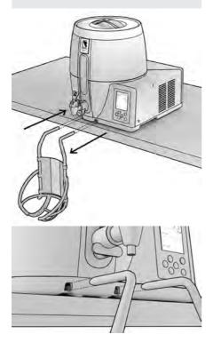
2. Remove the yellow dust cap from the keg liner and FIRMLY screw on the Connector as shown.
