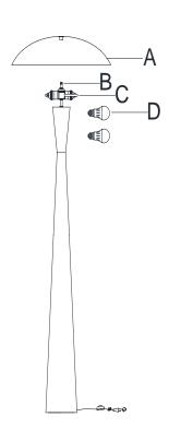
1. Thread Shade (A) onto the Rod (B) by turning clockwise direction until tight.
