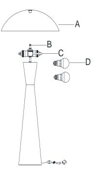
Thread Shade (A) onto the Rod (B) by turning clockwise direction until tight.
