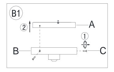
Remove Mounting Plate (A) from Canopy (B) by removing Canopy Screws (C).
