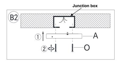
Attach mounting plate (A) to ceiling Junction box with mounting screws (O) provided.
