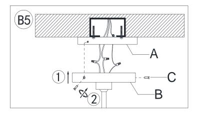
Attach canopy (B) to the affixed mounting plate (A) and secure with canopy screws (C).
