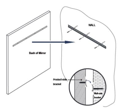
7) Mount the item to the wall by engaging either of the product-side brackets (according to the orientation you wanted) with the wall-side bracket, and then gently lowering the item so it rests on the wall.
