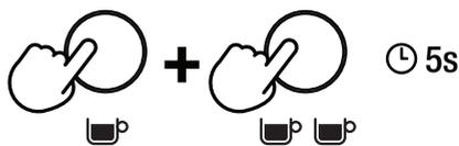
6. Press and hold the 1 CUP and 2 CUP buttons for 5 seconds to enter the cleaning cycle mode.
