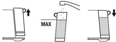
Replace the water tank onto the machine, ensuring it is properly attached and sitting flush against the back of the machine.
