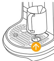
**5** Ensure the milk jug is making contact with the temperature sensor located in the drip tray.
