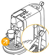
**2** To accommodate smaller cups, use the cup support. PUSH the cup support to unlock.
