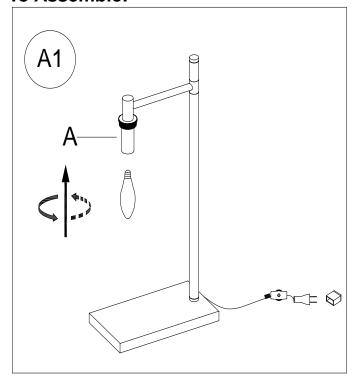
Insert one (1) **40-watt maximum TYPE B light bulb** (not included) or one (1) **9-watt compact fluorescent light bulb** (included for California customers only) into the Socket (A). DO NOT EXCEED THE SPECIFIED WATTAGE.
