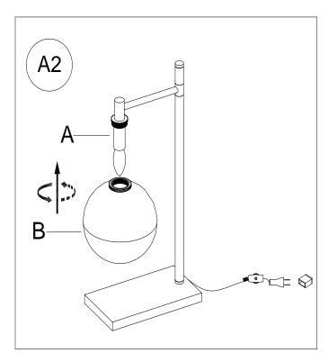
Attach the Lamp Shade (B) onto the threaded portion of Socket (A); secure the Lamp Shade (B) by turning the Lamp Shade (C) in a clockwise direction by hand until secure.
