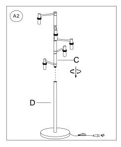
Thread the bottom nipple of Upper Pole (C) into the top opening of Lower Pole (D) by turning in a clockwise direction by hand until tight.
