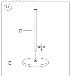
Screw Lower Pole (D) onto the center nipple of Lamp Base (E) by turning in a clockwise direction by hand until tight.
