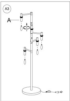
Insert five (5) **40-watt maximum TYPE B light bulbs** (not included) or five (5) **9-watt compact fluorescent light bulbs** (included for California customers only) into the Sockets (A). DO NOT EXCEED THE SPECIFIED WATTAGE.
