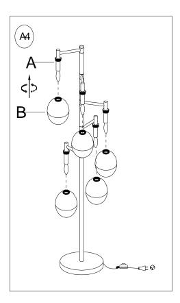
Attach the five Lamp Shades (B) onto the threaded portion of Sockets (A); secure the Lamp Shades (B) by turning the Lamp Shade (B) in a clockwise direction by hand until secure.
