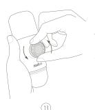
Unlock the piston from its travel position by rotating it to the left.
