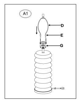
Raise the Harp Caps (E) and insert the bottom ends of Harp (D) into the Saddle (G)
