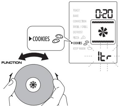
Turning TEMPERATURE/PIZZA SIZE/SLICES/TRAY dial (M) is possible to select "1tr" mode (1 tray of biscuits) or "2tr" mode (2 trays of biscuits).
