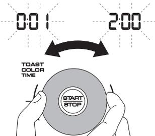
Press the START/STOP button (H) to start cooking. The red ON light (I), that is located around the edge of the START/STOP button (H), turns on.
