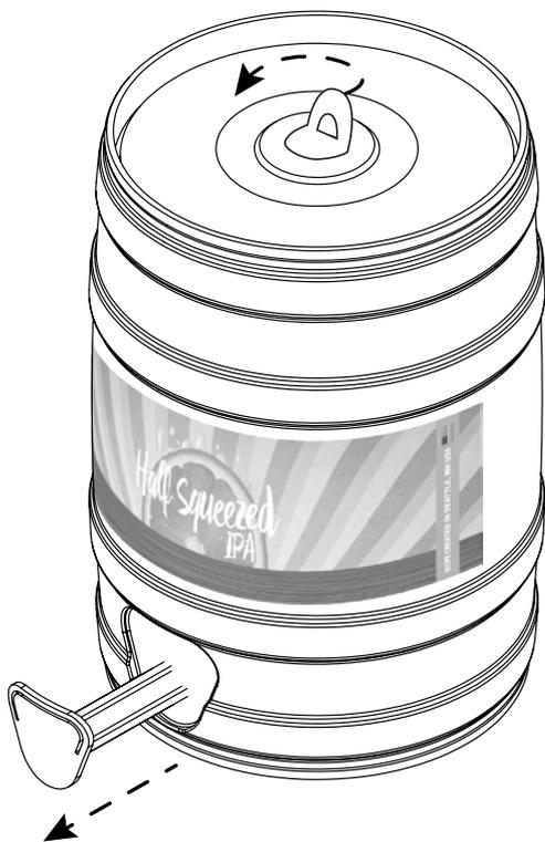
**2** Twist the Serving Keg Spout **counter clockwise** to dispense beer from the keg. Twist Serving Keg Spout **clockwise** to stop dispensing beer.
