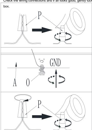
Connect the GROUND FIXTURE WIRE to the GROUND J-BOX WIRE using the Plastic Wire Nut Connector (P) and wrap the connection with electrical tape. Be sure that no wire strands are exposed.
