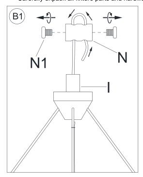
1. Loosen set screws (N1), pull out the safety cable from lock connector (N).
