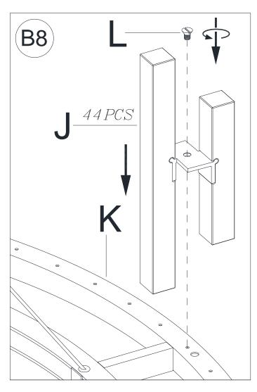
10. Loosen the Set Screws (L), then place the Brackets (J) onto the Light Fixture (K) and secure the Brackets (J) by tightening Set Screws in a clockwise (L)
