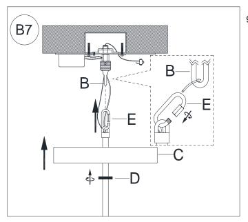
Attach Hanging loop (E) to Mounting Loop (B)
