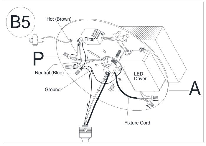
7. Connect the wires from Filter with the wires from the ceiling junction box. Connect the fixture cord with the wires from the LED Driver.
