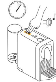
**2 To enter the descaling mode**, ensure the machine is ON, press and hold the 3 coffee buttons for 6 seconds until the confirmation with a beep. The 3 buttons will start blinking (buttons will flash until the exit of this mode).
