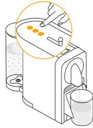
**7 Press any button to start** descaling a second time. Machine will stop automatically when the water tank is empty. Empty and rinse the water tank, drip tray and cup support thoroughly to avoid any residue.
