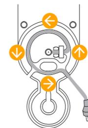
**2** Adjust the cable length and store the excess under the machine. Insert the remaining cable in the guide under water tank left or right socket, depending on the position chosen for the water tank. Ensure machine is in the upright position.
