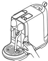
**5 Dry all the parts** with a repetitive soft clean cloth and reassemble all parts. Clean the coffee outlet and inside the machine regularly with a clean damp cloth.
