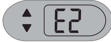
The mixer is equipped with a self-resetting safety device which safeguards against overheating the motor with excessive loads. If overheating occurs, the mixer will automatically activate the overheating protection device and the motor will switch itself off. If this error occurs, turn the speed control dial to the 'OFF' position, and unplug the cord. Wait at least 15 minutes before restarting the mixer.
