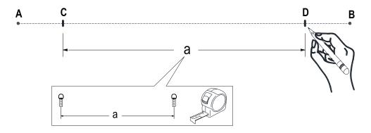
Use a stud-finder to determine if there is a wall stud[s] located at [each] either insertion mark.
