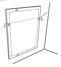
Connect the two points (A, B) with a light pencil line. Use a level to ensure that the line is level.
