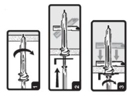
**Tips:** The toggle is self-drillable. No pilot hole required.
